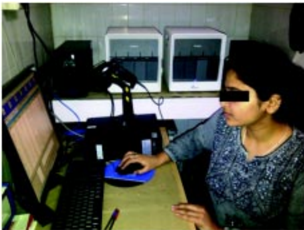
Fig 2 — Xpert® MTB/RIF (Cepheid Inc, Sunnyvale, CA, USA), an Automated 2-hour Test for TB and Rifampicin Resistance
