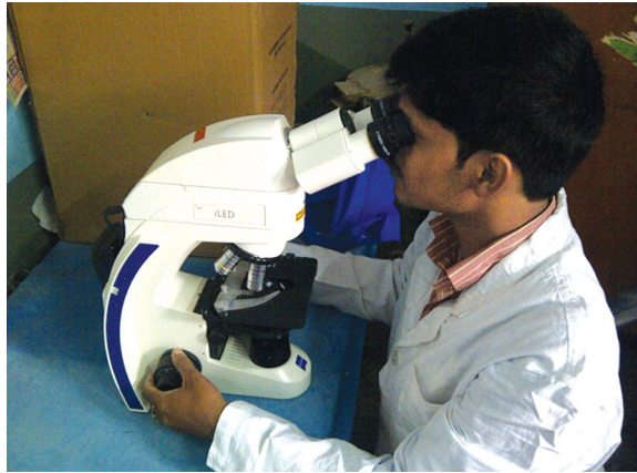
Figure 1: Light-emitting diode fluorescence microscopy for acid-fast bacilli.
